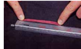
Becoming "forgetful": Highly stressed over time, both rubber band and mesh filament relax or elongate and become incapable of full recovery to size.
