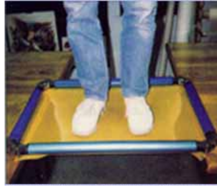
Forceful statement: A screen tensioned to 50 N/cm easily holds the weight of a grown person.
