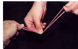
Key word is "tends": Like the rubber band, the individual mesh filament tends to recover its original shape and size when deflected.
