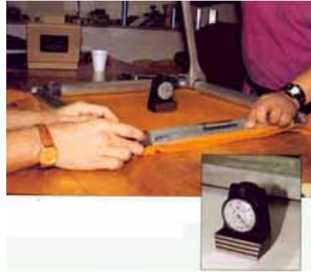
Printers' " hearing aid ": Once the screen is recognized as your ink-transfer mechanism, it's easier to appreciate the importance of elevated tension. The inset shows the reward of careful tensioning.
