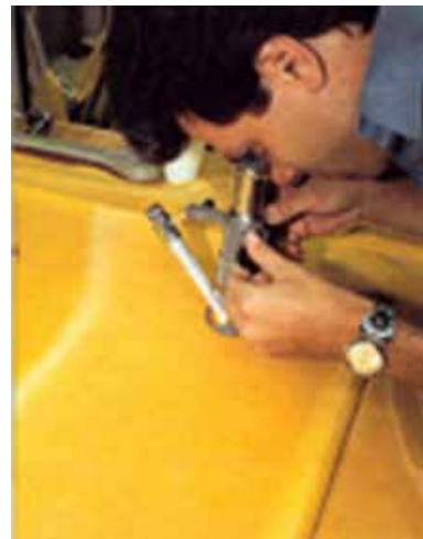
The nitty-gritt: Observing the effects tension has on mesh with the aid of an illuminated, 100X loupe enables this technician to assess his results on the filament level .
